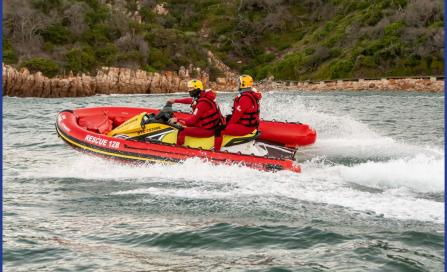
In early 2019, Admiral Powercats and Droomers Yamaha approached the NSRI with a design concept for a jet boat, a jet ski with an extension hull and hypalon pontoon permanently attached. It seemed to tick all the boxes for an exceptional surf rescue craft and in July 2019 the prototype, given the Sea Rescue class name JetRIB, was taken on a tour of Sea Rescue stations around South Africa.
